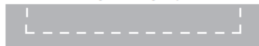
Continuous parking bay adjacent to the kerb (words may be added outside the bay to describe the type of parking)
